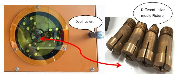
Select the corresponding product diameter mold, install the mold, adjust the clamping length, turn on the air source, and adjust the depth of the groove.
