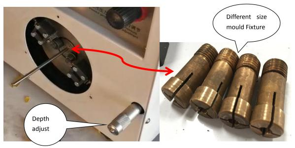
Select the corresponding product diameter mold, install the mold, adjust the clamping length, turn on the air source, and adjust the depth of the groove.
